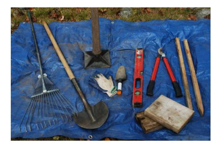
**Tools for resetting a stone**Rake, shovel, tamper, gloves, level, loppers,
